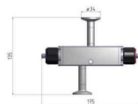
Sampling head with 2 clamps DN 10 DIN 32676 Ø 34 mm
